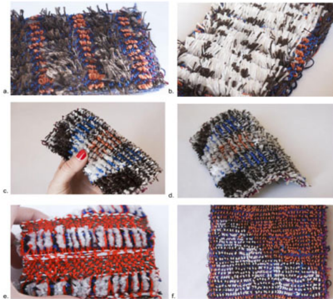
Figure 17: Jacquard pile samples: (a) cut and looped pile stripes (b) varied length directional pile (c) cut and looped pile with Jacquard graphics (d) same (e) cut pile stripes (f) looped pile with varied ends and Jacquard graphics. © VTRG 2019. Photos: Emily Holtzman.
