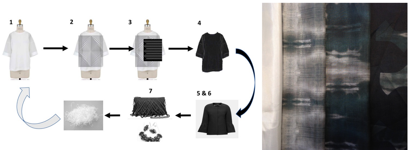
Figure 6: Left – planning out the shirt overprint and remanufacturing sequence to communicate to the partners in the research consortium. Right – the ‘Ikat’ print sample series showing the build-up of tone-on-tone.
