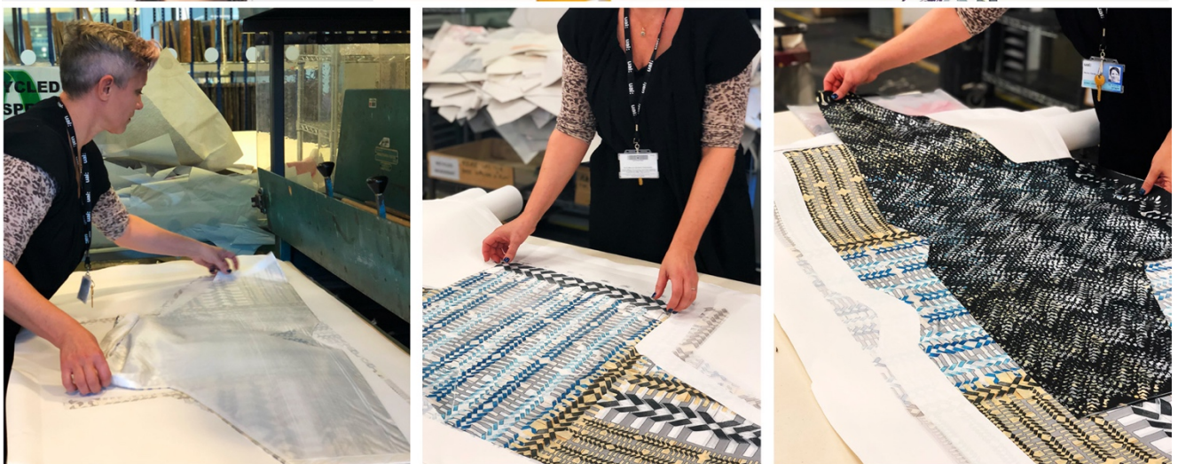
Figure 7: Left and centre – The researcher printing the first shirt with the digital dye sublimation design. Right – the second overprint shirt, on top of the first overprint and plain shirts.
